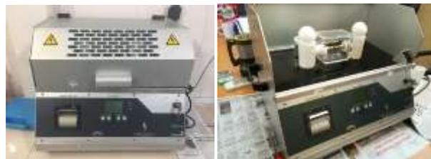
Gambar 9. Alat Penguji Tegangan Tembus Type Portatest A2
