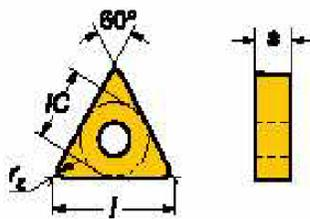
Figure 1. CBN Sculpting Geometric Description:  $r = 0.8$  mm;  $iC = 12.7$  mm;  $S = 3.18$  mm;  $l = 16$  mm
