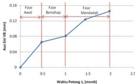
Figure 5. The curve of relationship between side wear VB vs time cut  $t_c$  at  $V = 267$  m / min,  $a = 0.7$  mm, and  $f = 0.125$  mm / rev
