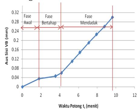
Figure 2. The curve of the relationship between side wear VB vs time cut  $t_c$  at  $V = 200$  m / min,  $a = 0.3$ mm, and  $f = 0.1$  mm / rev.
