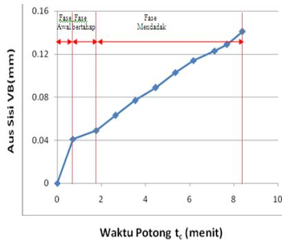
Figure 4. The curve of relationship between side wear VB vs time cut  $t_c$  at  $V = 225$  m / min,  $a = 0.7$  mm, and  $f = 0.1$  mm / rev
