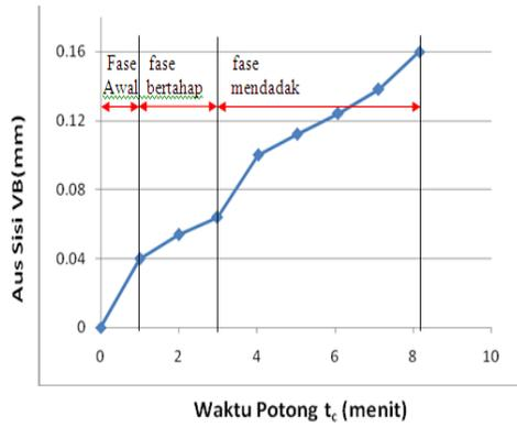
Figure 3. The curve of relationship between side wear VB vs Cut Time  $t_c$  at  $V = 200$  m / min,  $a = 0.3$  mm, and  $f = 0.15$  mm / rev
